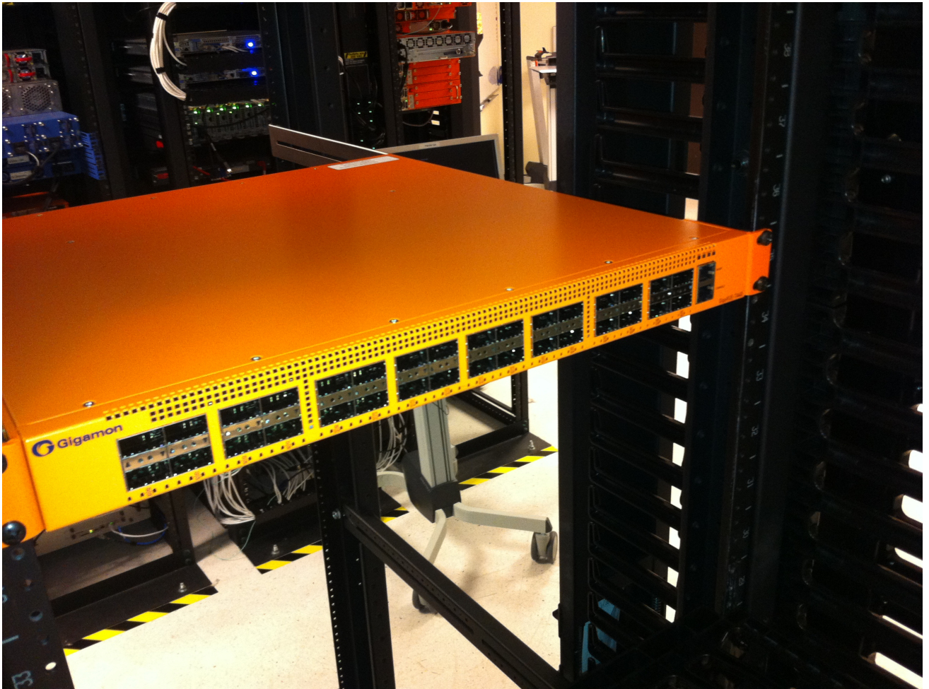
Figure 5 Front View of the Mounted Node to the Four-Post Rack
